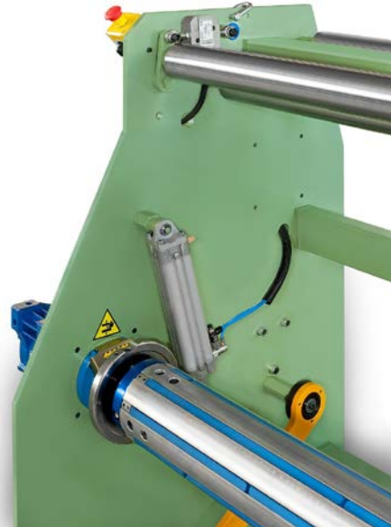
Winding tension control by load cell and pressing roller
